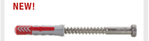
Standard Wall mount (included in the wall to center rail): M8 cylinder head bolt ZK8.100.HD with wood thread, Fischer-UX Ø 10 mm, 80, 100 and 120 mm
